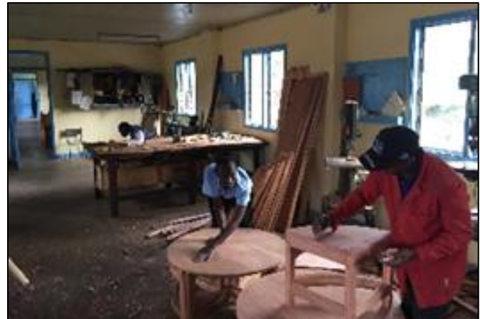
A coffee table with stools/nest of tables under being made by the students
