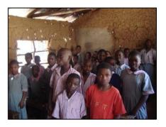
The old classrooms were built of mud and wooden poles with no windows. Over time the walls are eroded by rain. Floors are compacted earth.
